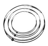
DRAIN PANS AVAILABLE IN 22" (559 mm) DIAMETER (PART NO. 66001011) FOR WATER HEATERS HAVING A DIAMETER 20" (508 mm) OR LESS, 24" (610mm) DIAMETER (PART NO. 66001105) FOR WATER HEATERS HAVING A DIAMETER 22" (559 mm) OR LESS AND 28" (711 mm) DIAMETER (PART NO. 66001012) FOR WATER HEATERS HAVING A DIAMETER 26" (660 mm) OR LESS.
